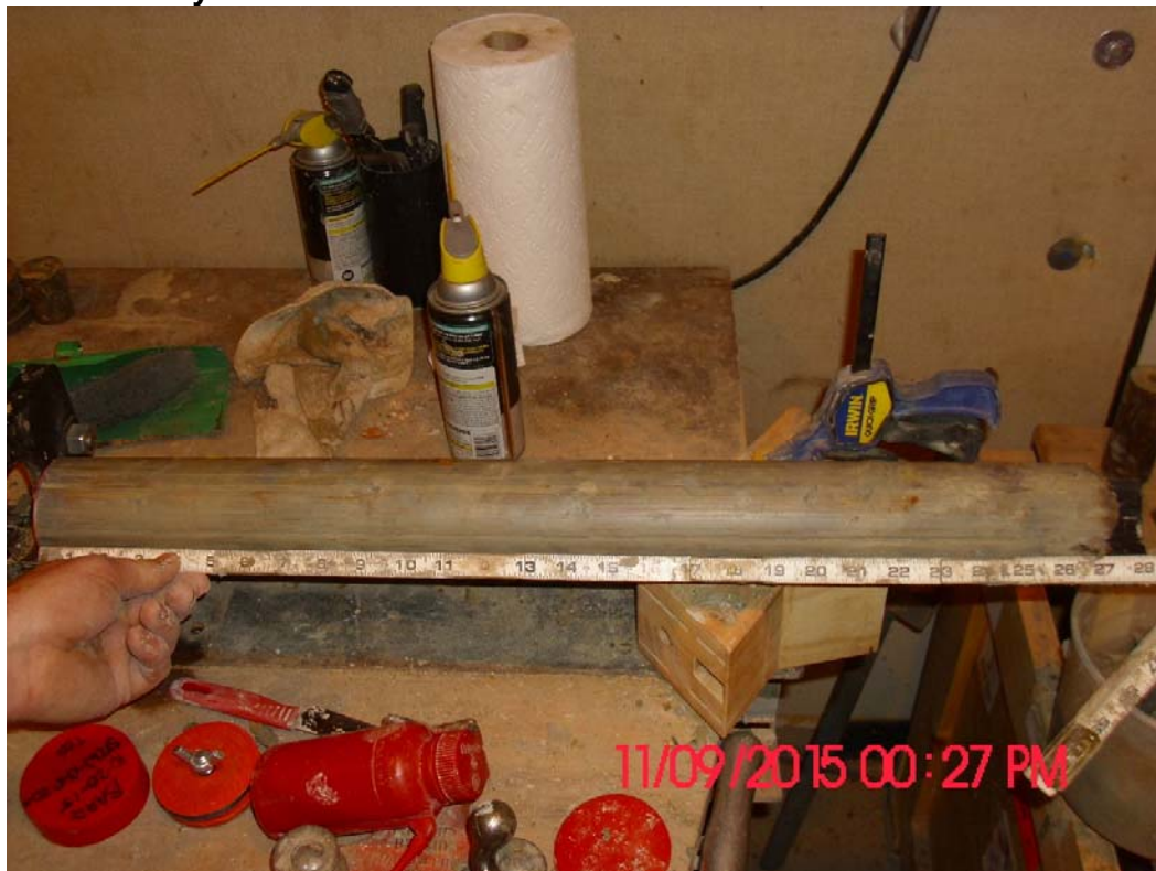
Photograph 8 – East Scrubber Pond Liner sample extruded from Shelby tube prior to testing
