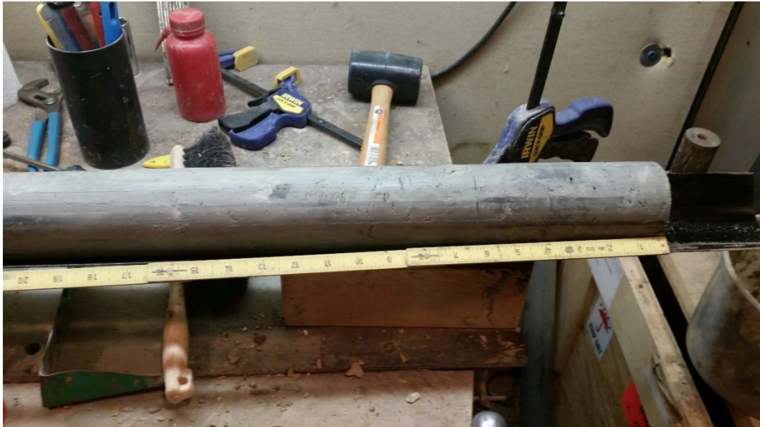
Photograph 4 – West Scrubber Pond liner sample extruded from Shelby tube prior to testing
