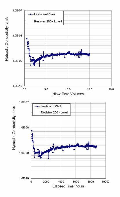
Permeability with pore volumes and time for the Resistex® 200 FLW9 GCL using site specific leachate per ASTM D6766, Scenario II, for the Montana Dakota Utility, Lewis and Clark CCR Scrubber Ponds
