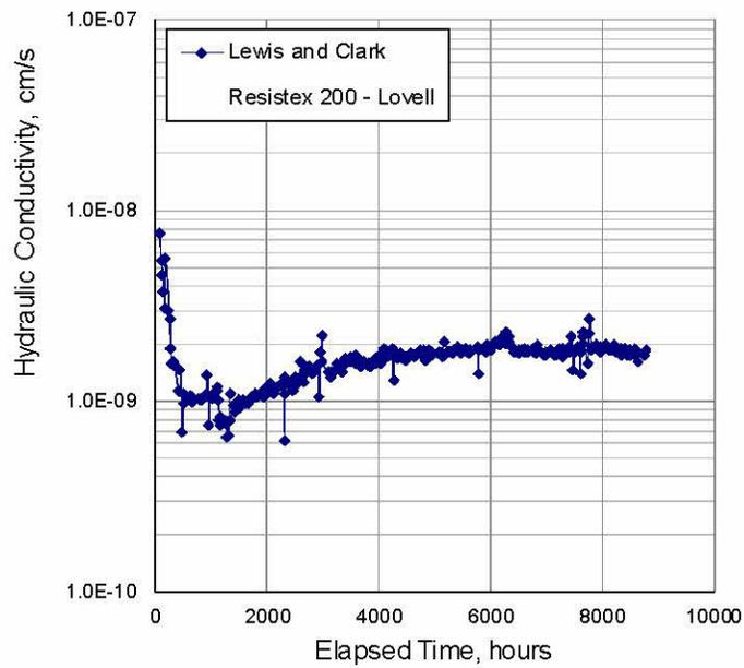
Permeability with pore volumes and time for the Resistex® 200 FLW9 GCL using site specific leachate per ASTM D6766, Scenario II, for the Montana Dakota Utility, Lewis and Clark CCR Scrubber Ponds
