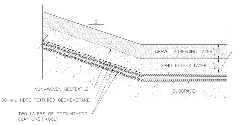
FIGURE 1 TYPICAL LINER SECTION LEWIS AND CLARK STATION MONTANA-DAKOTA UTILITIES BISMARCK, ND
