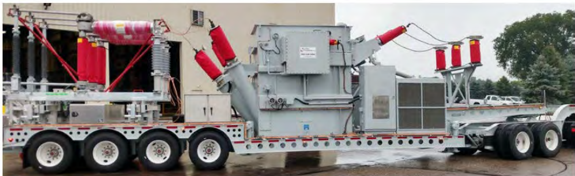
12 13 Figure 7 – Mobile Distribution Substation Example
